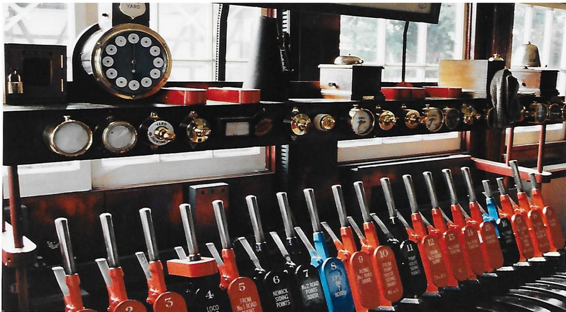
5. The levers in the signal box are connected to which pass along the track and connect to rods alongside the track which actually operate the points. These rods can be seen in the photograph below.
