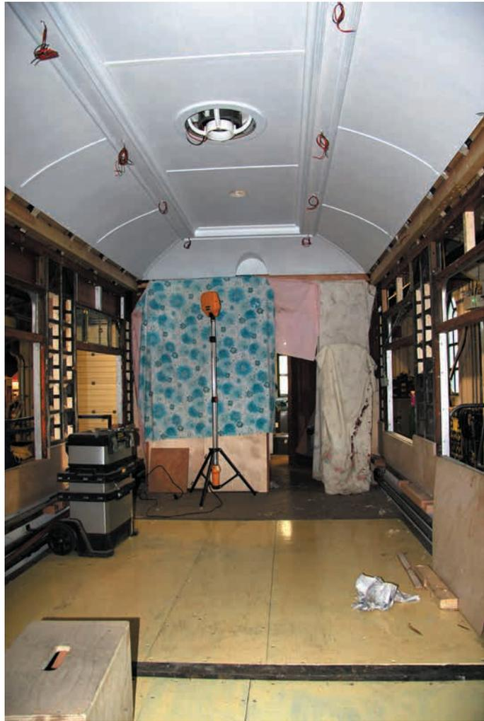
Car 54's northern saloon is progressing well. Painting of the ceiling is well advanced and rags used to protect the marquetry panelling that couldn't be removed. Ply panelling has been fitted under the sidelights and the steam heat pipes installed. French polished panels and decorative heater guards will cover them in due course. DAVE CLARKE
