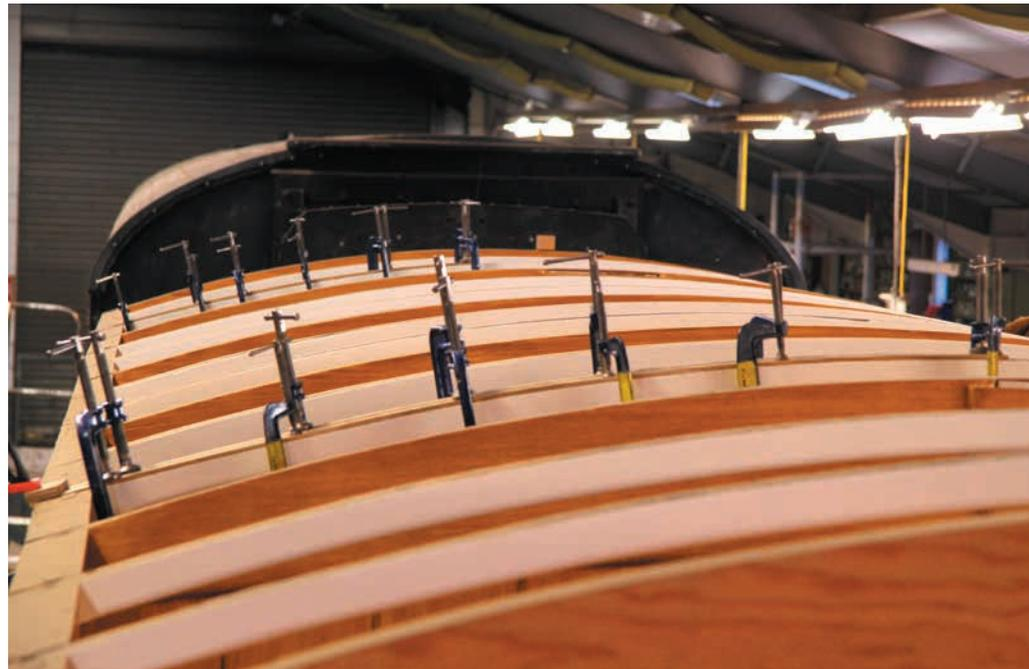
Timber strips have been attached to the east side of a couple of LBSCR Third No 328's roof hoops. They will be pared back to produce a more uniform roof profile when the roof boards are fitted. DAVE CLARKE
