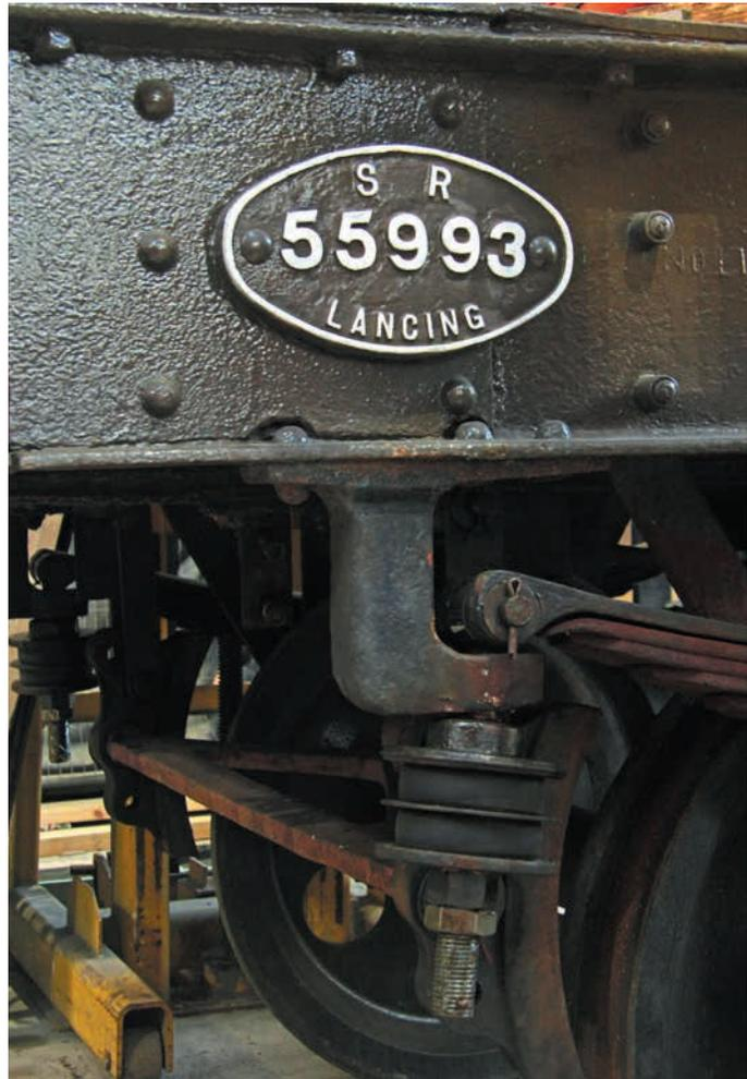
Eight newly fabricated, steel I-bolts, have been fitted to SR Pillbox Van No 55993. They are attached to the end of the spring by a large pin, which is secured with a split pin. It then passes through the 'J' bracket, which is riveted to the van's frame, a collar. A couple of rubber disks and some spacers follow before a couple of nuts are added to secure them in place. DAVE CLARKE
