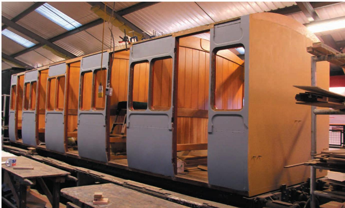
The panelling on the east side of No 328 is now in a uniform shade of grey. Most of the mouldings have yet to be fitted to the cant and bottom rails and the lower part of the mid rail down the length of the coach. DAVE CLARKE
