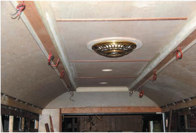
The decorative mouldings have been applied to the wiring trunking and the first cover strips installed over the joins between the ceiling panels of Car 54's southern saloon. The central ceiling fan cover has been temporarily fitted, the other holes are for ceiling lights and ventilators. DAVE CLARKE
