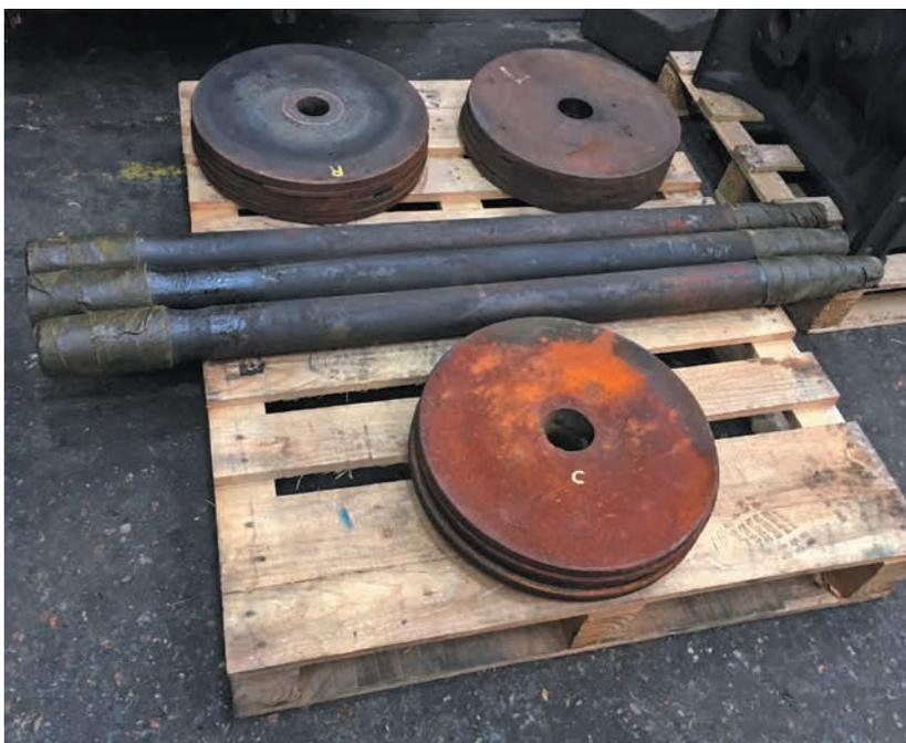
Piston heads removed from Stowe's piston rods.
