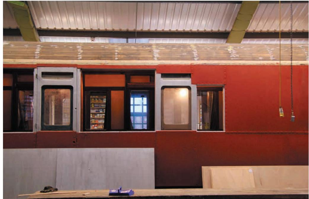
Red oxide primer has been applied to the steel panelling on the east side of SR Corridor Brake Third No 3687. A peculiarity of Maunsell corridor coaches is that half the six doors along the corridor are non-operational dummies, the partially-clad 'A' compartment 'door' on the right is one of these. The new, narrow roof board has been fitted above the cant rail and all holes in the roof filled in readiness for canvassing. DAVE CLARKE
