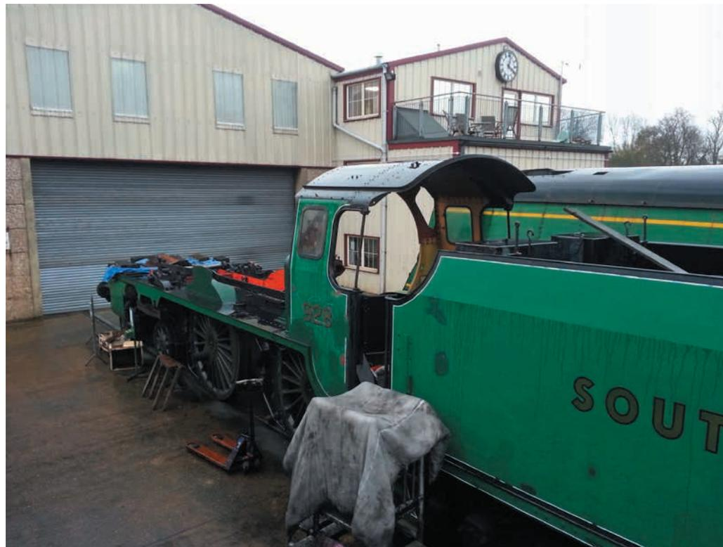
Stowe's new cab roof in place on the cab sides on 4 March. STEVE PILCHER
