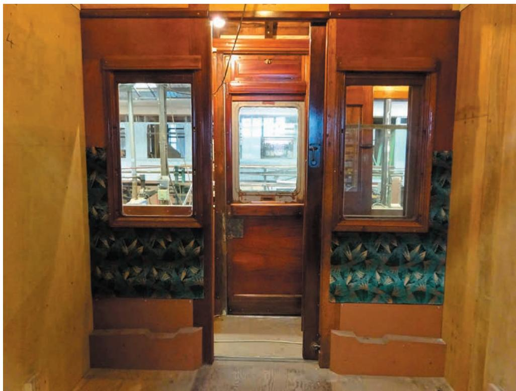
The fit-out of No 3687's Compartment F is under way. The white glossed bulkhead partition tops can just be glimpsed. The varnished mouldings and blind boxes have been fitted to the corridor partitions along with the green 'jazz' quarter panels. ALEX MORLEY
