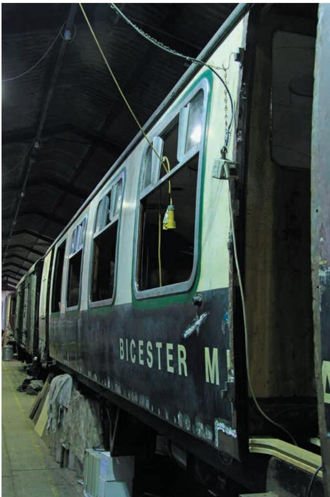
The sidelights have been removed from the west side of Mk.1 TSO No 4754. After any corrosion induced repairs, paint was applied around the edges of the surrounding panelling. This has enabled the refurbished frames and fixed toplights to be returned to the first three apertures. DAVE CLARKE
