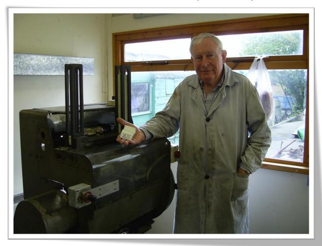
The Bluebell Railway bought two and after restoration one was brought into service in May 2006 producing all the Bluebell tickets. It was manufactured in 1941 and up to August 2013 more than 1 million tickets have been produced by the machine which is located at Sheffield Park in a small shed at the rear of Platform 1. The machine is designed to print on blank tickets, pre-cut to the standard Edmondson ticket size of 21/4 inches by 13/16 inches, (57.15mm x 30.16mm).
