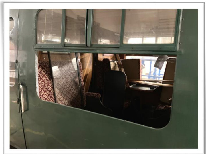
Above: 1482 with one of its main lights removed for new seals to be fitted, 3 April 2024
