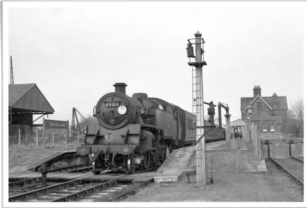
BR Standard 4MT 2-6-4T No. 80011 heads the 12.28 p.m. East Grinstead to Lewes service at Sheffield Park on 16 March 1958, the day before BR closed the line. Note the signal post in place but has no semaphore arm.
