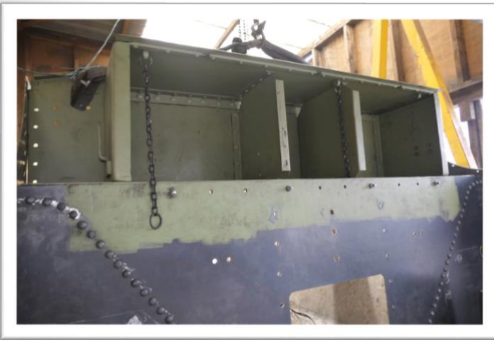
Left: The original tender toolboxes have been renovated and are now back in place at the front of 541's new tender tank. Photo: 4253 Group.
