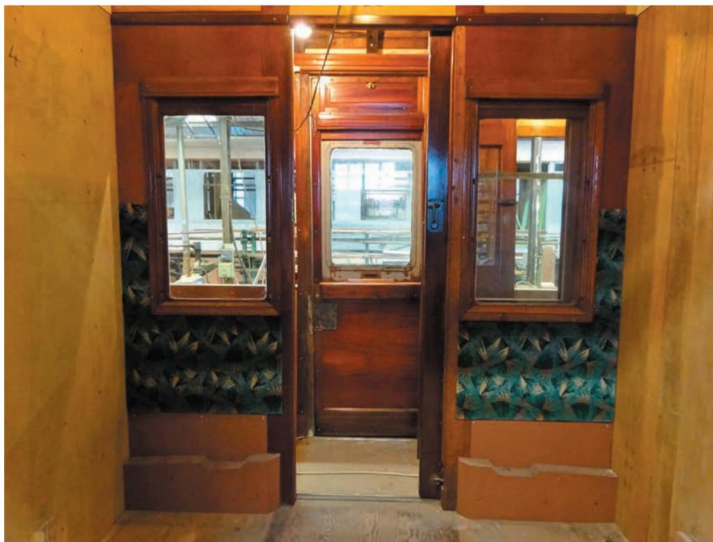
The fit-out of No 3687's Compartment F is under way. The white glossed bulkhead partition tops can just be glimpsed. The varnished mouldings and blind boxes have been fitted to the corridor partitions along with the green 'jazz' quarter panels. ALEX MORLEY
