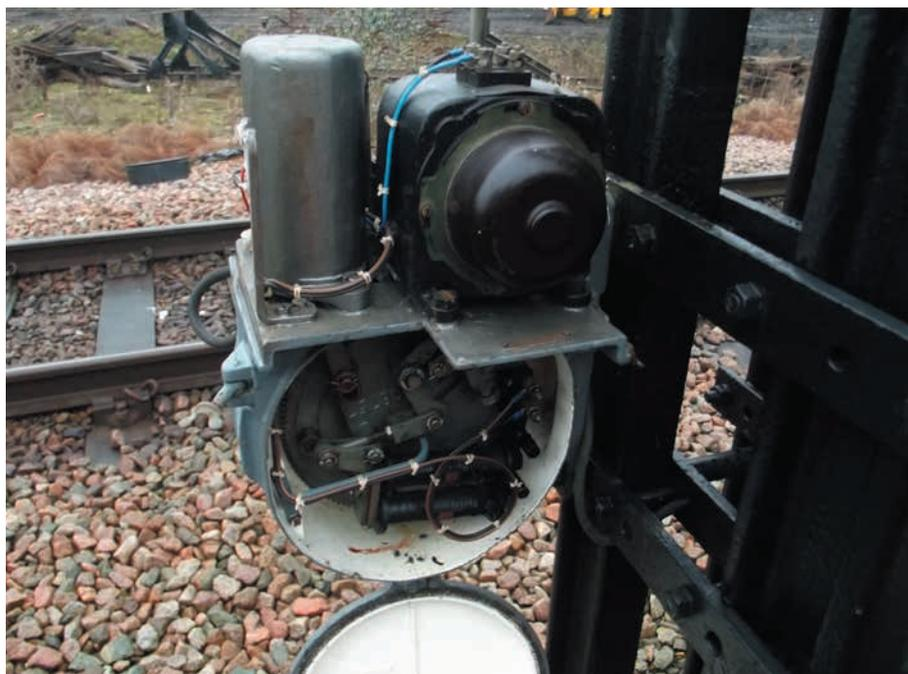
A signal Machine (circa 1927) with its covers removed. Top right is the electric motor, top left an air damper to slow the fall of the arm, below is the gearing and hold off mechanism. BRIAN HYMAS
