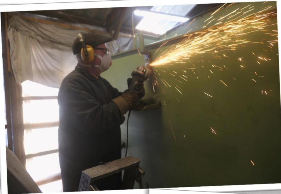
Left: Grinding down rivet heads on tender lamp irons
