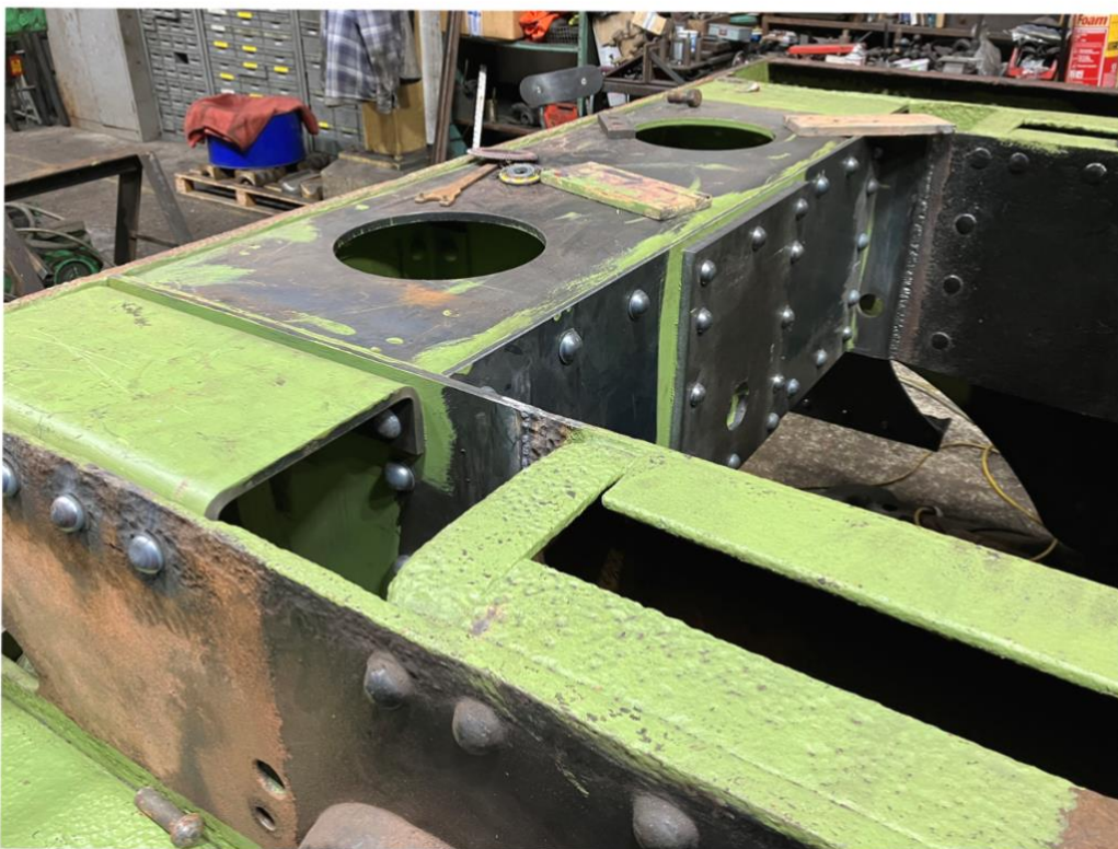
Left: 541 tender new rear drag box fabrication rivetted in place
