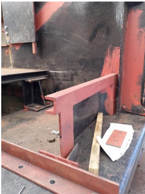
Cab floor supports under construction and shovelling plate in final position
