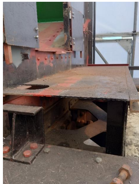
Cab floor supports under construction and shovelling plate in final position
