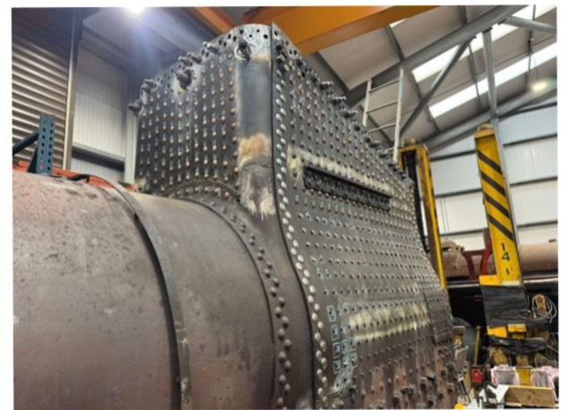
Top: A view of the inner firebox, showing the new copper stays and new monel stays with their stay nuts fitted.
