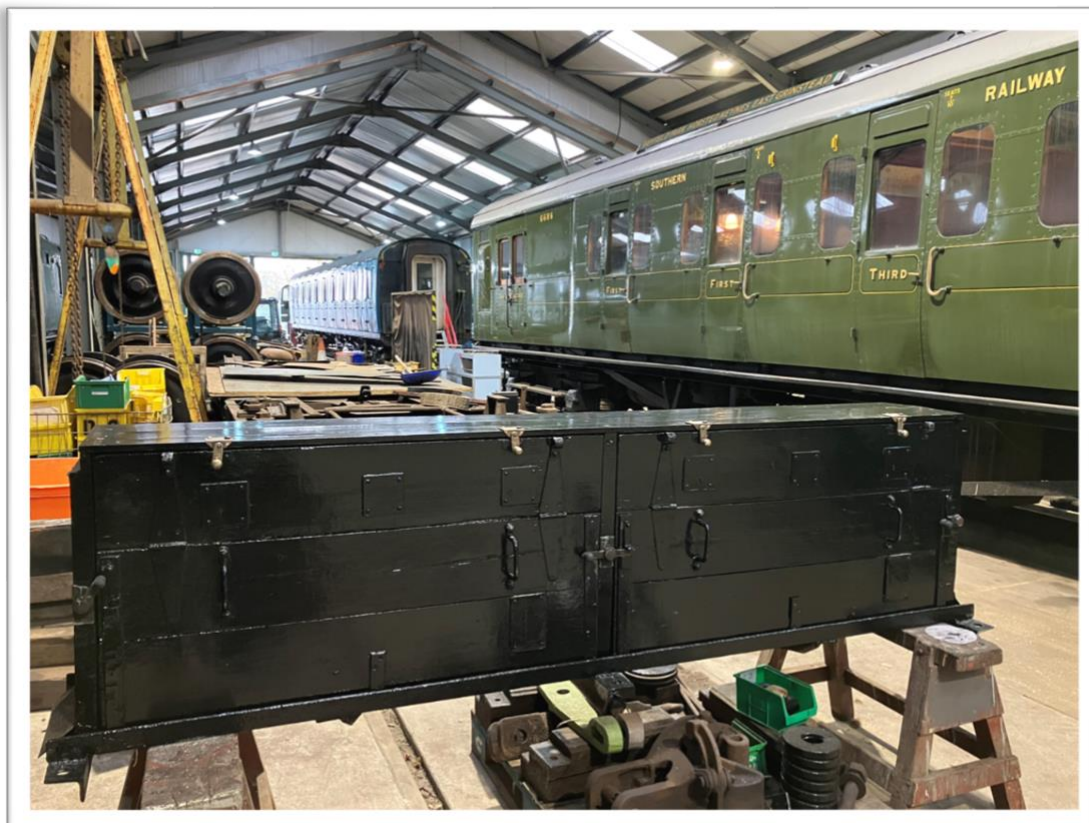
Below: The completed west side battery box. 6 Dec 2025
